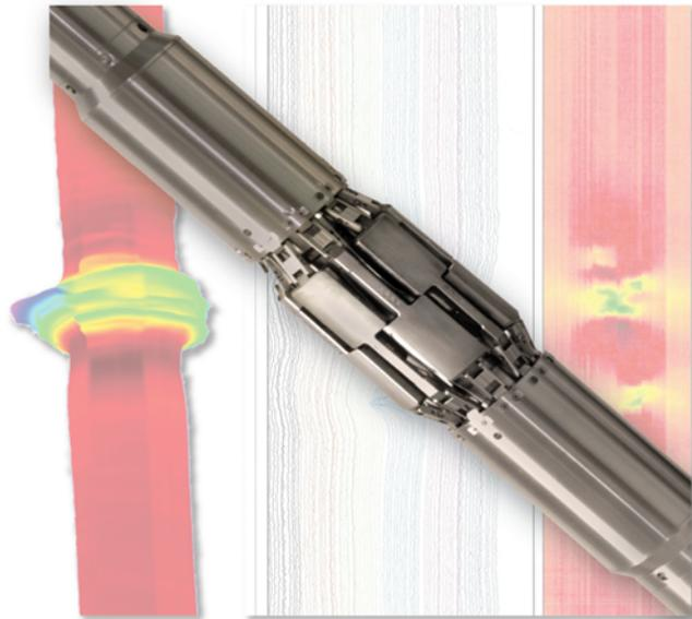
Depending on casing size, the MFL sensor section has 8 to 16 pads. Each pad has 8 magnetic field sensors for measuring the magnetic flux leakage independent of logging speed, and two shallow discriminator measurements to determine if the measured flux leakage is internal or external. Together with a high speed memory section, the CIT provides the highest resolution 3D image of the integrity of the casing.
